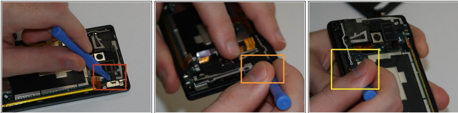
**⚠** This step involves removal of the top camera and speaker module. **Read the next two steps before starting**, as it is easy to rip one ribbon cable if you pry the part too far
