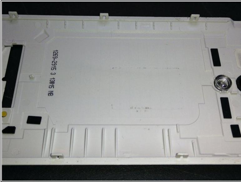
! Take care not damaging the thin coating off the rear case as shown in the picture of the white version of the ZL.
